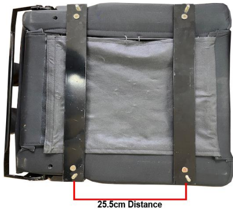
PHOTO(A) Note front conversion plates welded bolts position
