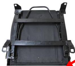
\*For an easier fitment, wedge in a flat head screw driver between the track and handle to slide and position the "U shape" handle over the locating pins
