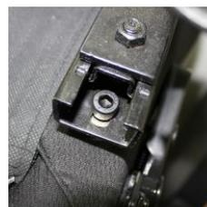
5. Place the assembled seat onto the original seat mounting holes by using the 4 original bolts and washers. In some vehicles, larger washes are needed. Washes not supplied. Tighten all bolts to correct manufacturer tension.\* Attach the removed seat belt to the adaptor seat belt bracket with the provided bolt and nut/washers and secure correctly.
